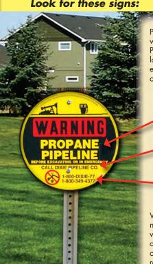
Pipeline markers can be found along the right-of-way and where the pipeline intersects a street, highway or railway. Pipeline markers are used to indicate the approximate location of the pipeline - do not rely on them to indicate the exact position of the pipeline as it may not follow a straight course between markers.
